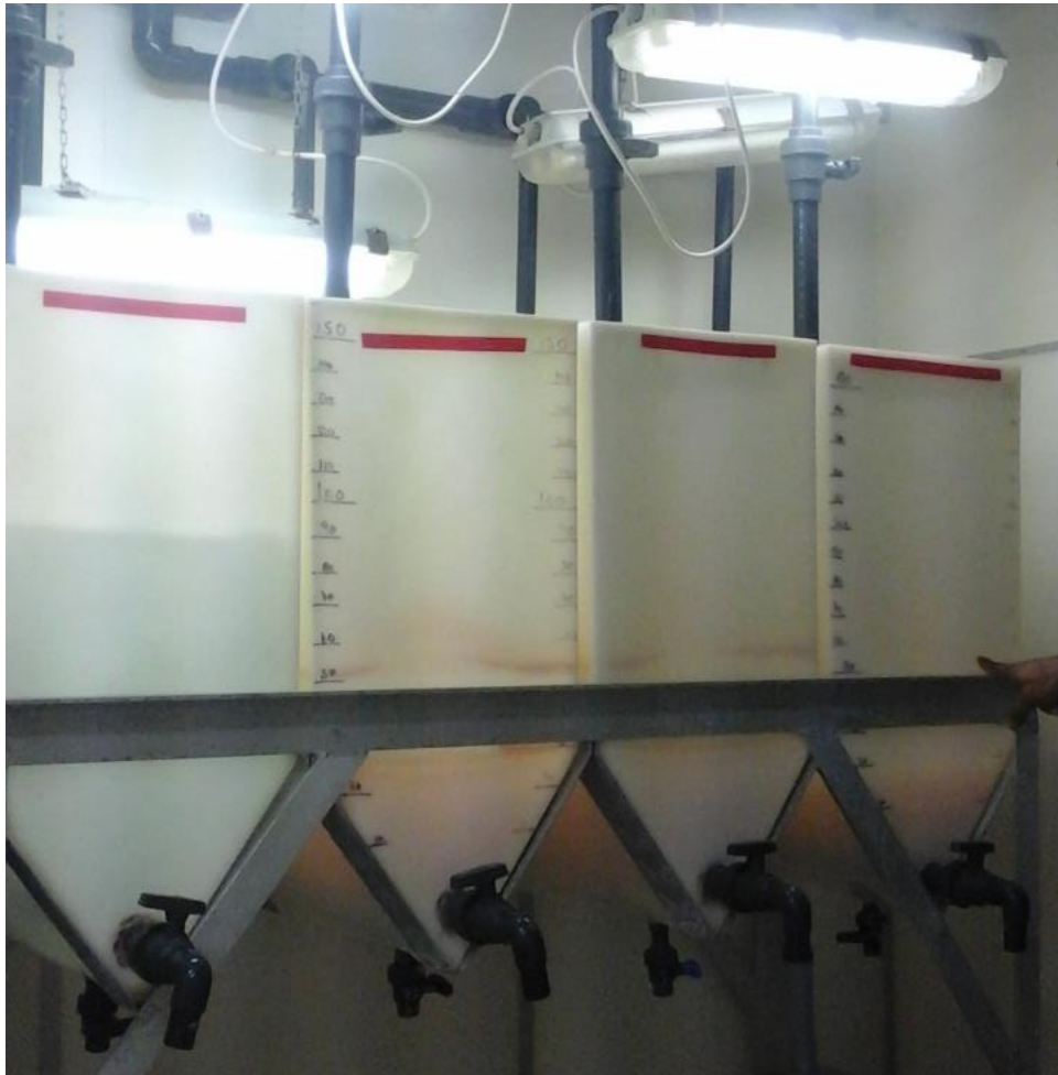
Figure 10. Enrichment tank with 50L of water per tank
